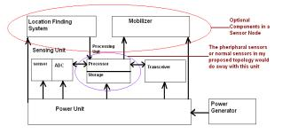
Fig.3.The components of a sensor node [2]
