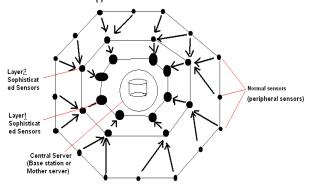
Fig.1. Proposed Heterogeneous Wireless Sensor Network
